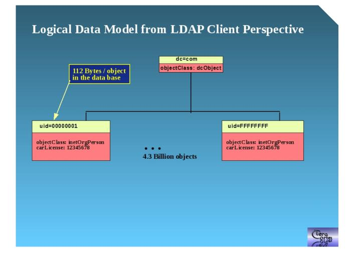
Figure 3: Logical data model (client perspective)
