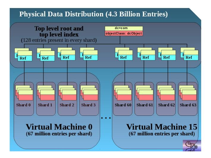
Figure 4: Simplified physical data model (server perspective)
